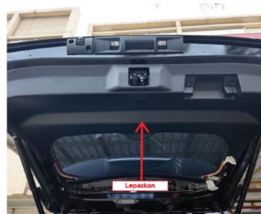
3. Lepas panel trim pintu bagasi (tailgate/power back door).
