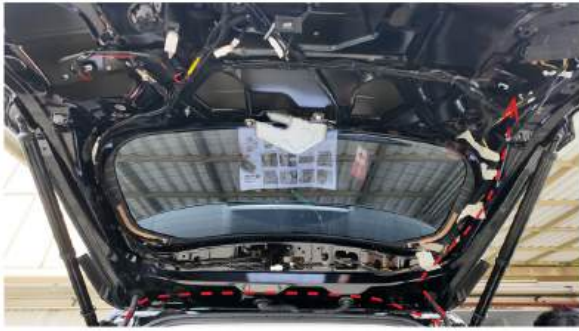
17. Masukkan power harness ke power tailgate.
