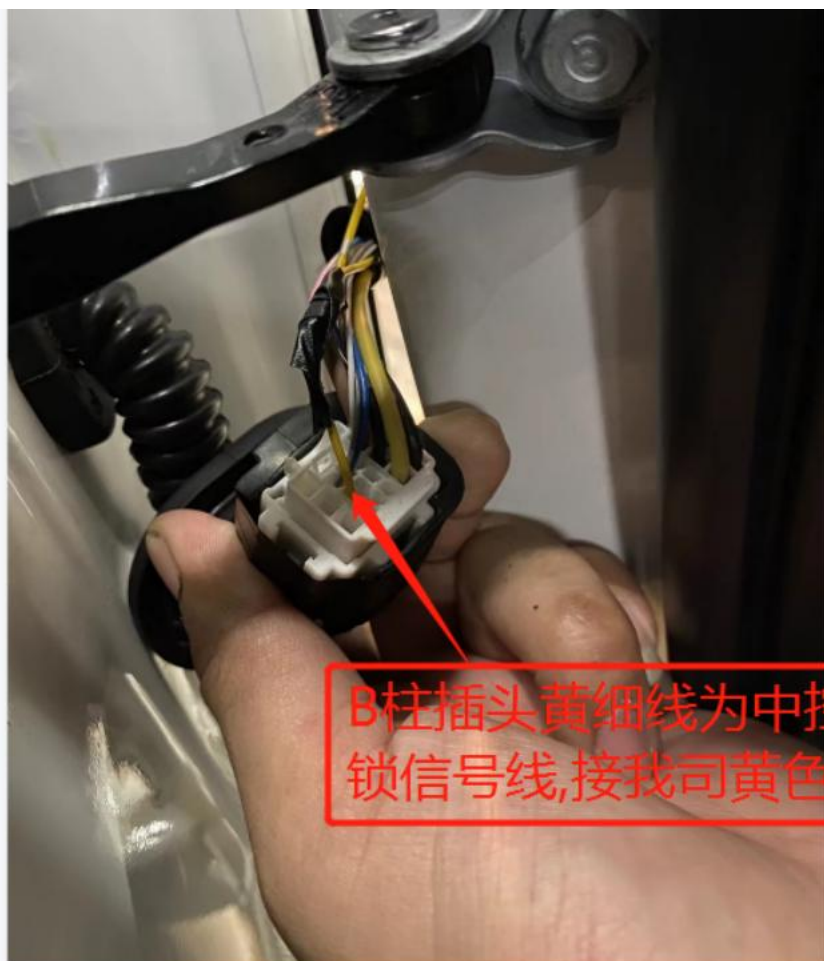
11. The thin yellow cable of the B-pillar plug is the central control release cable.
