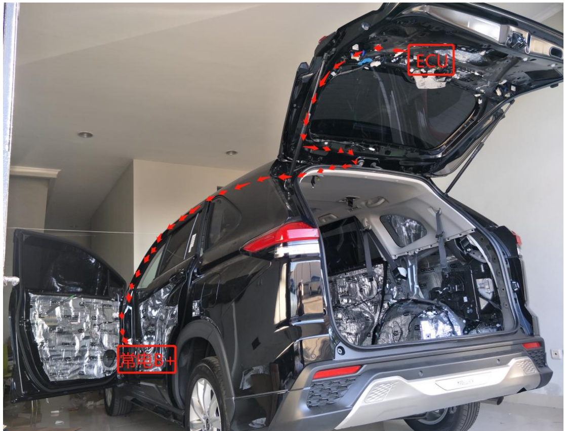
18. Location for ECU and location for B+.
