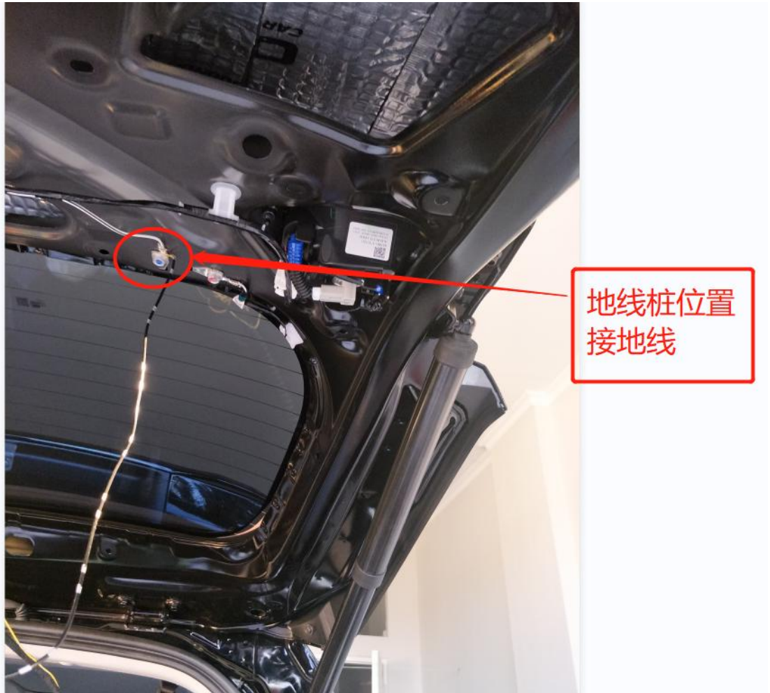
12. Location for GND,it is important.
