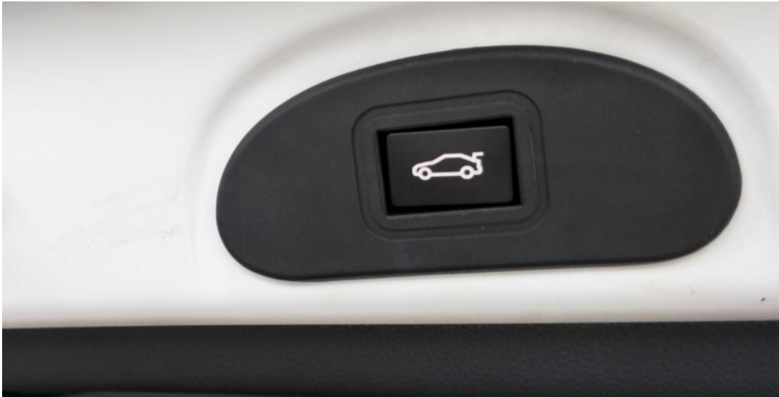
25. Rear Switch installed.
