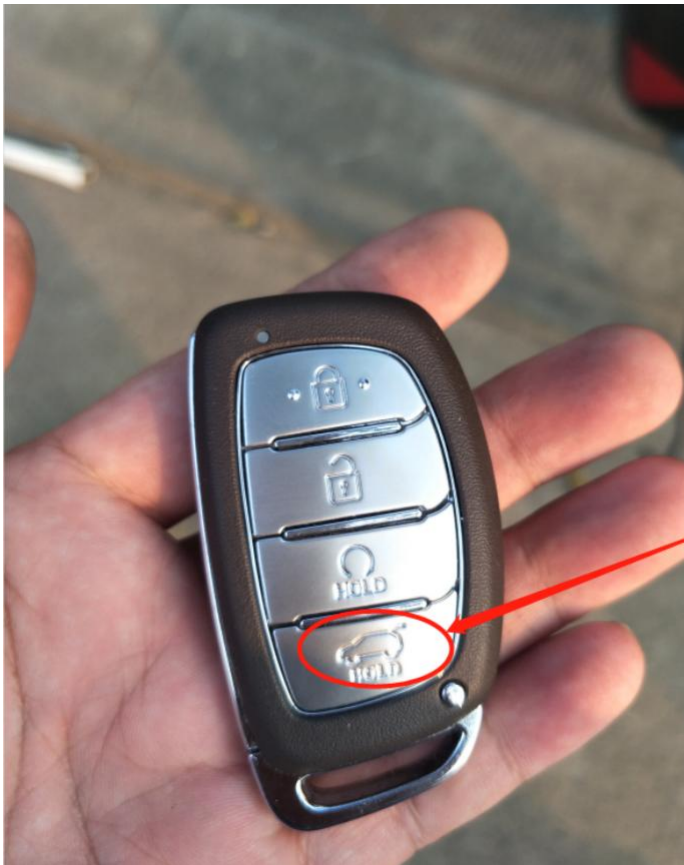
26. Pressing "trunk" button on original key two seconds to open or close the trunk.
