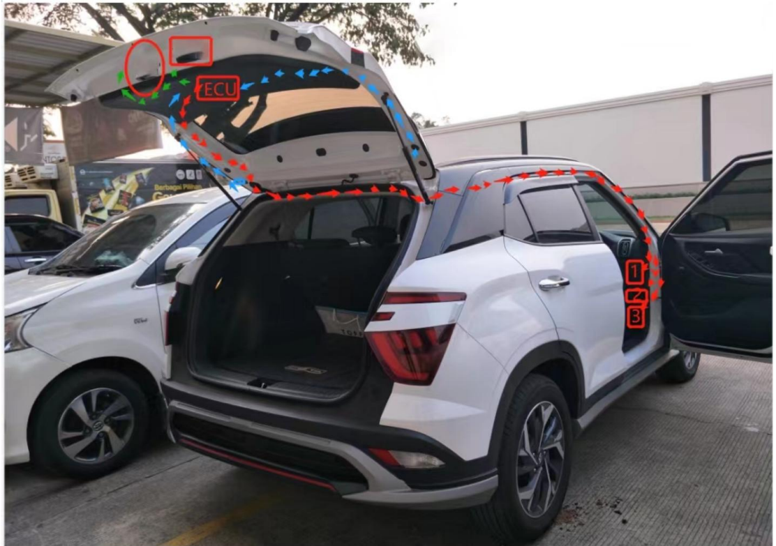
15.Red arrow show the power cable/CAN cable/front switch wiring.
