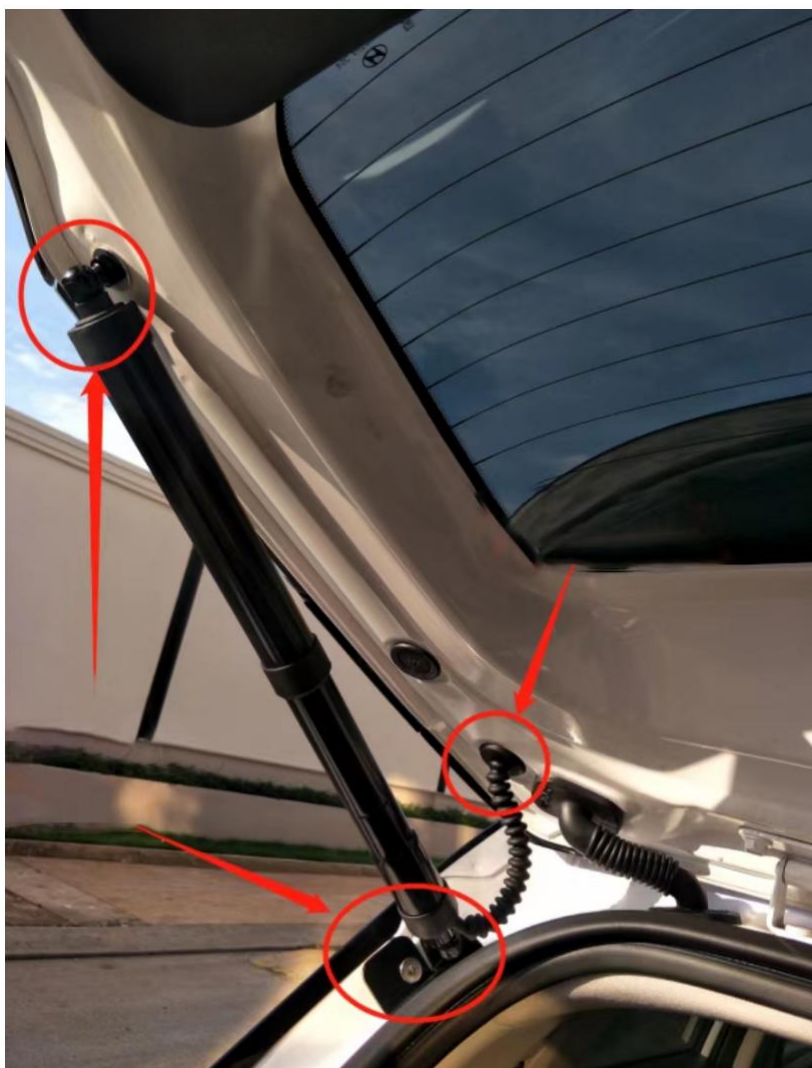
8. Install the electric strut and cross the strut line.
