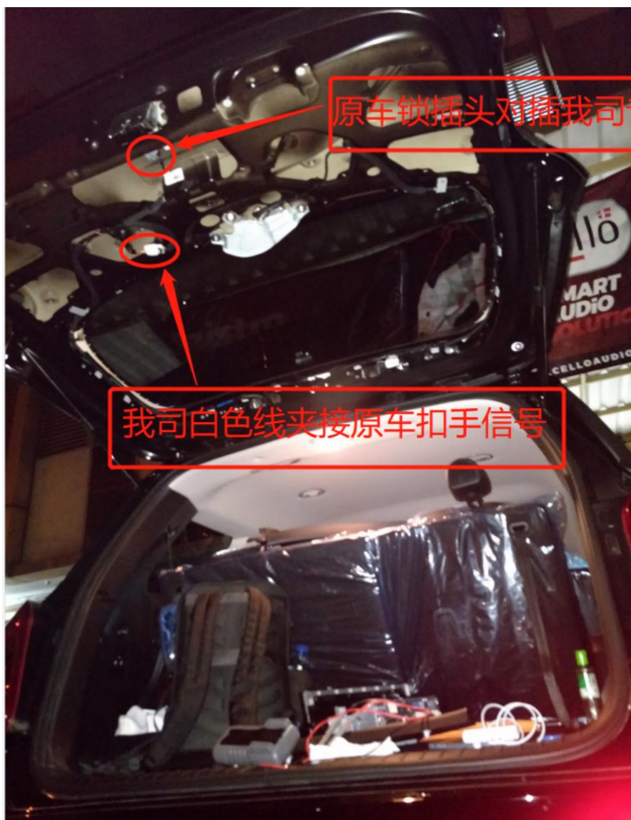
13.The original car lock plug is inserted into our special plug.Our white wire clip the original car lock hand signal line.
