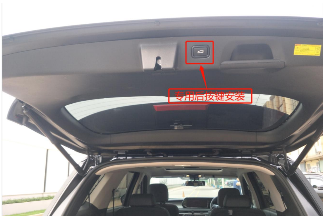
25.Rear Switch installed.
