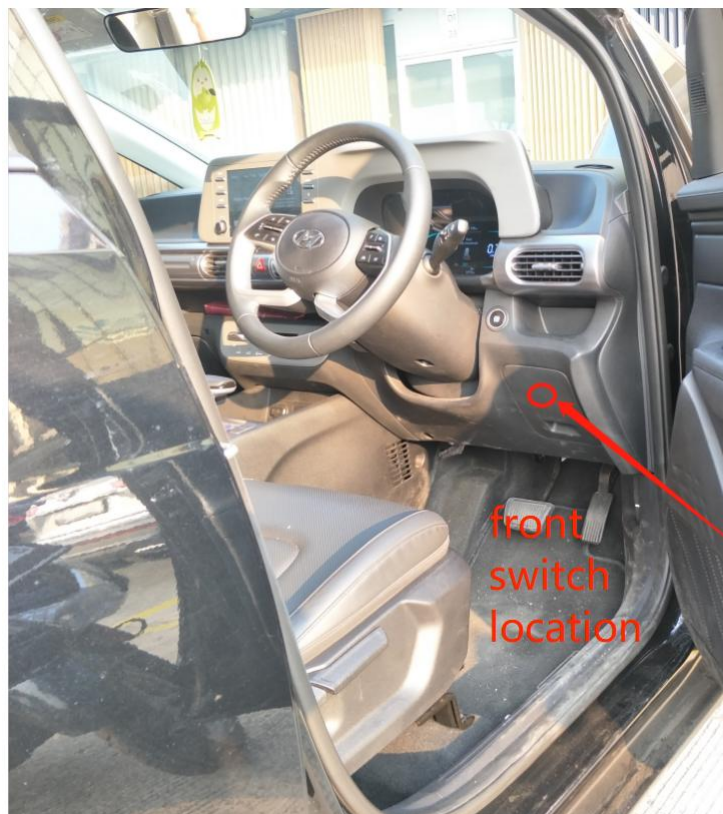
18. Location for front switch.
