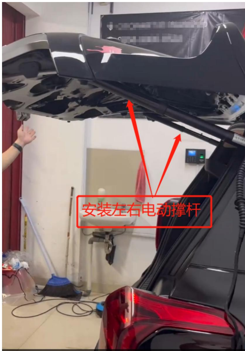
9. Install the left and right struts.
