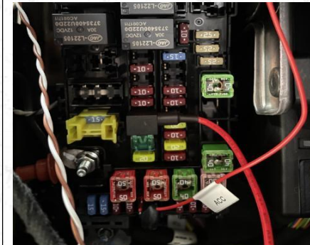
8.Find the original car safety box, take 12V normal electricity
