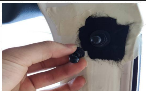
5. Remove the original tailgate ball head and install our company equipped with ball head (the left and right are the same)
