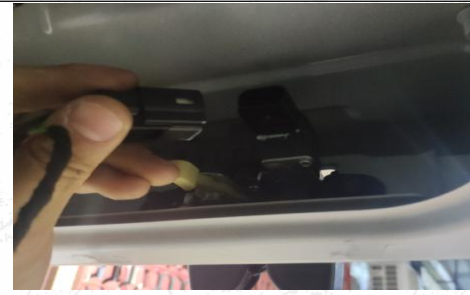
8. Unplug the original car lock plug and connect it with our wiring harness
