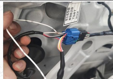
10. Our white line is connected to the original car's white hand buckle signal cable
