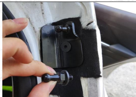
4. Remove the ball head of the original car body, install our body bracket, and use our screws ("L" is the left and "R" is the right)
