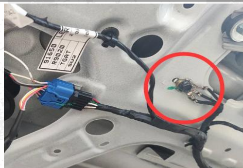
9. Power supply negative tower iron position
