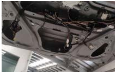
4. Remove the main trim of the tailgate
