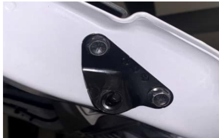
6. Remove the tailgate bracket (same left and right)
