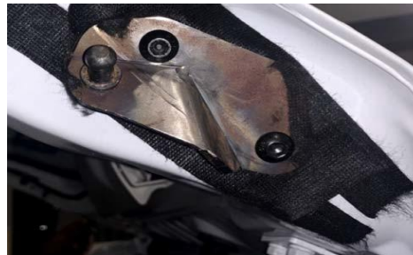
7. Use our original car screws to install our tailgate bracket ("L" left "R" right)
