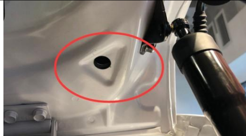
9. Use a 16mm drill to make holes in the position of the tailgate picture (same left and right)
