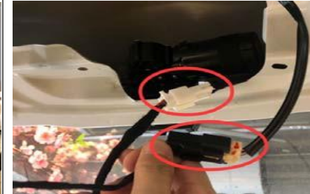
12. Unplug the original car lock wire and connect with our wire
