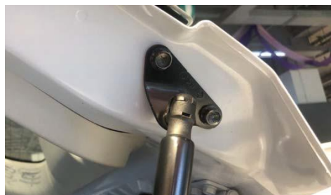
5. Pry open the gas spring snap ring and remove the original car brace (same for left and right)
