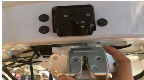
11. Remove the original car lock and install our electric lock
