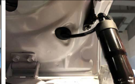
10. Thread our strut wire into the hole and plug the rubber plug (same left and right)
