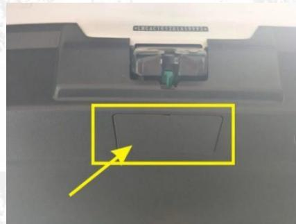
**!** When the tailgate cannot be opened normally, find the original car emergency safety lock in the trunk, open the emergency cover and pull the emergency switch to open.
