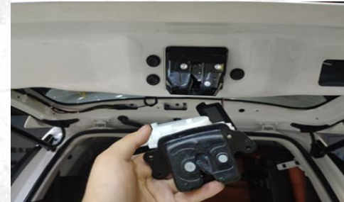
9. Remove the original car lock and install our upper suction lock
