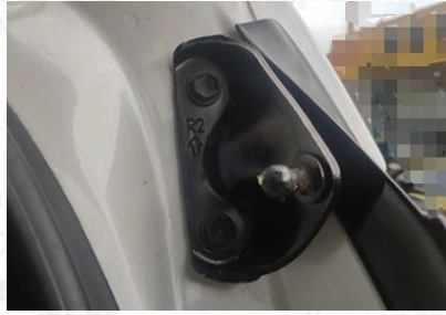
4. Remove the original body bracket (same left and right)
