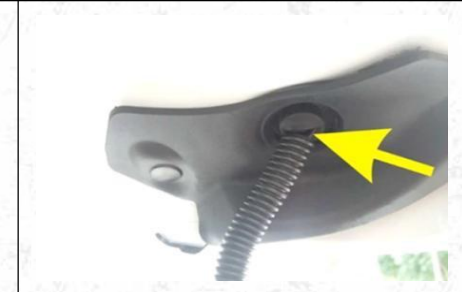
8. Pass the strut wire into the reserved hole and plug the rubber plug(same left and right)
