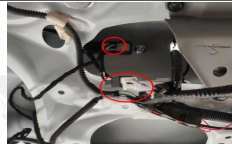
11. Unplug the original car lock wire and dock with our wire
