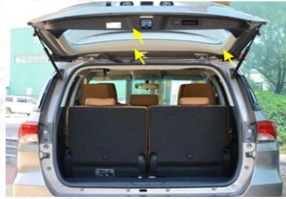
2. Remove the trim panel in the picture
