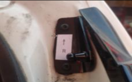
5. Install our body brackets ("L" left and "R" right)
