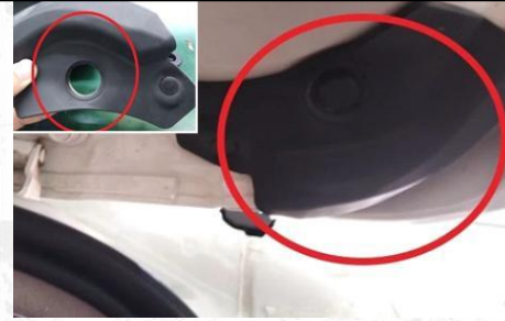
7. Cut the rubber plug of the original car (same left and right)
