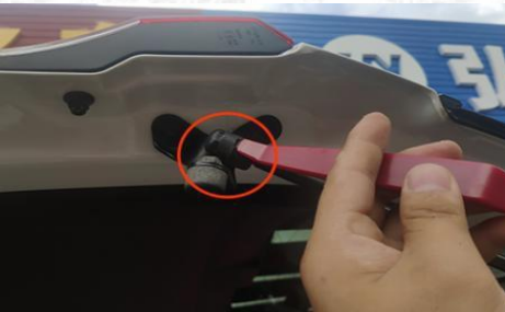
3. Pry open the gas spring snap ring and remove the original pole (same left and right)
