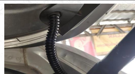
10. Put electric poles' wire through the hole then cover rubber plug, same left and right.
