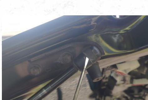
5. Using pry tool take off the jump ring and take out gas poles. same left and right.
