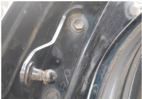
6. Take off the original bracket on car body. same left and right.
