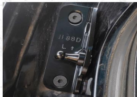
7. Install new brackets on car body.
