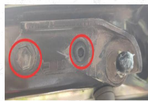
8. Use our screws instead of original screws ( still use original tail gate brackets )
